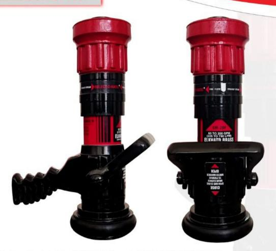
Nozzle Gun Protek Syle 333 Inlet Size: 1-1/2" OR 2-1/2 Multi Porpuse Nozzle with Pistol Grip. Cabable of flowing solid bore and FOG Stream Independently or both at the same time. Operates Effectively from 50 PSI (3.5 BAR), 75 PSI (2.25 BAR) tp 100 PSI (7 BAR). Exceptioanly lightweight and compact. Suitable for use with cafs system. Optional solid bore tips size 3/4", 7/8", 16/16", or 1". Inlet Size is 1-1/2" (38 mm), or 2-1/2" (65 M).
